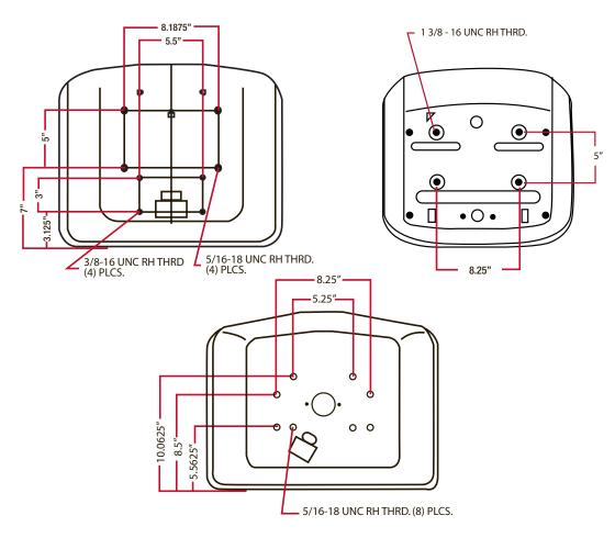
As this bulletin covers many different part numbers of seats, you will need to determine exactly what size bolts your specific seat and application will need. The threads will either be 5/16-18, or 3/8-16 and some seats could use either depending on which mounting bolt pattern used.
